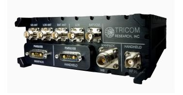
The **TCR-MBA-50-WB-Dual** is designed to support modern Handheld and Manpack Transceivers. The amplifier supports emerging Wideband Networking Waveforms including SRW and ANW2, as well as legacy Narrowband Waveforms such as IW, DAMA, SINCGARS and HAVEQUICK. Additionally, the amplifier integrates seamlessly into systems using new Special Communications Modes in both LOS and SATCOM.
